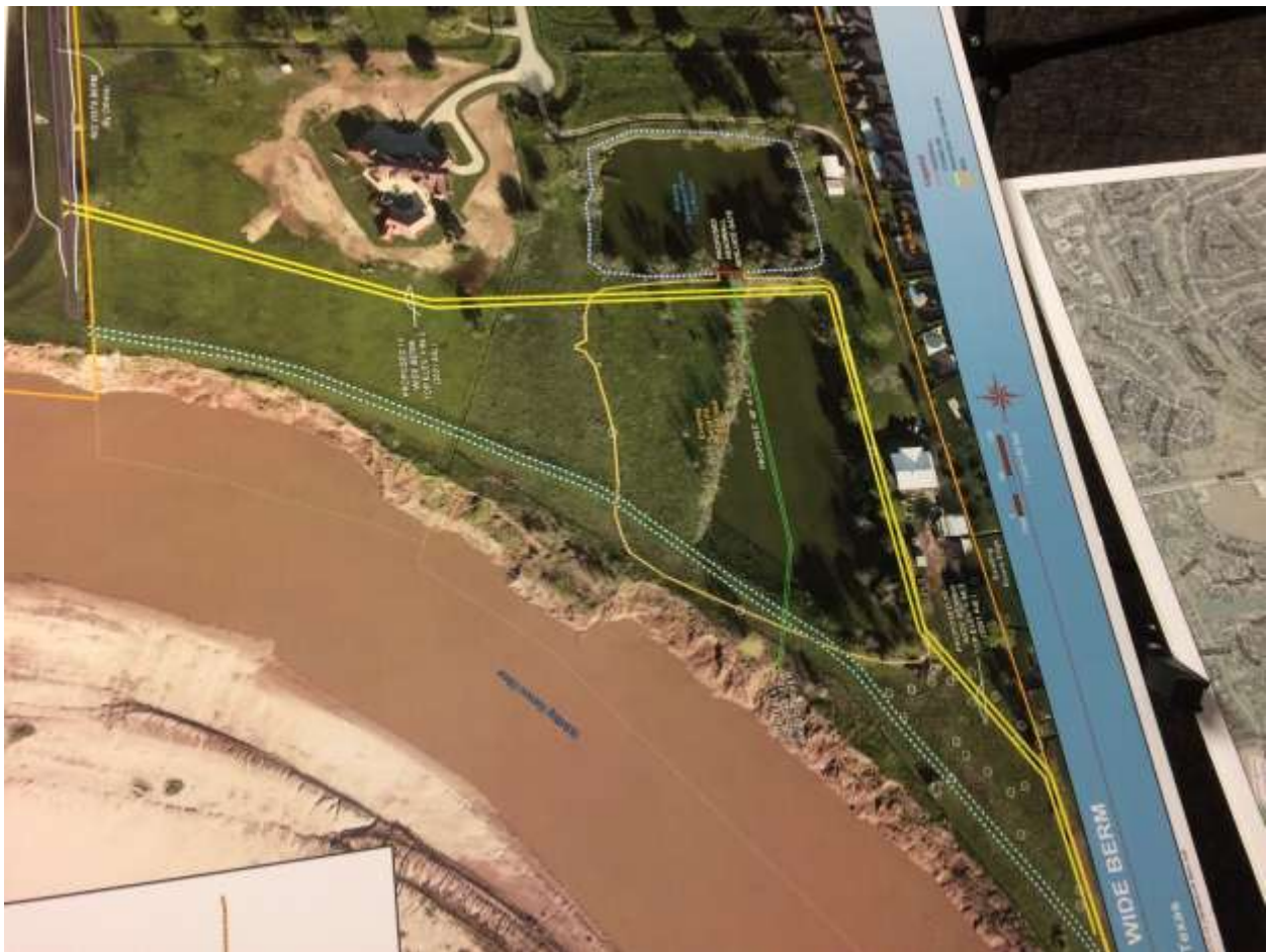
Old Berm (Double Dotted Green Line) and proposed New Berm (Double Yellow Line) at west end of DRS. Single yellow line shows pond which would be filled in.
